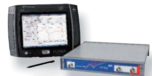
Vector Network Analyzer Bode 100 (1 Hz – 40 MHz) with Future.Pad Tablet PC from www.ibd-aut.com
